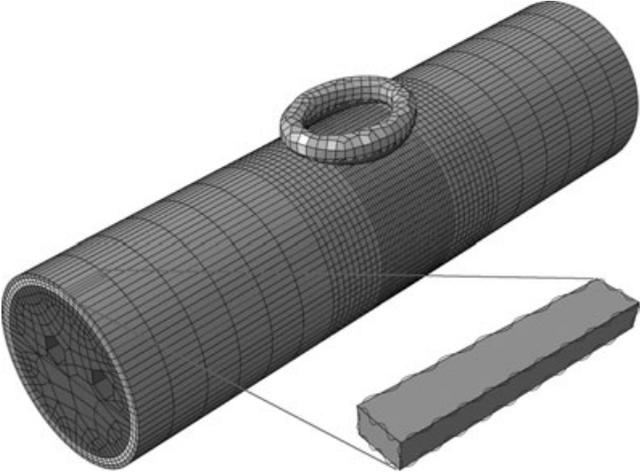
Fig. 3. Geometry and mesh of the FE model. Different tissue areas are indicated with different colours. The fibres are visualized as springs within the magnified element. The suction head consisted of 3063 and the tissues of 26137 elements.
