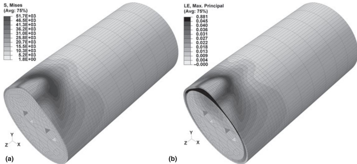
Fig. 7. (a) von Mises stress ( $S$ ) and (b) logarithmic strain ( $LE$ ) distributions in the forearm tissues at rest under 13.3 kPa suction pressure. The highest von Mises stress value (51.9 kPa) was located in the skin at the longitudinal ends of the stretched area. The highest logarithmic strain value (0.88) was located in the adipose tissue under the suction area of the skin.
