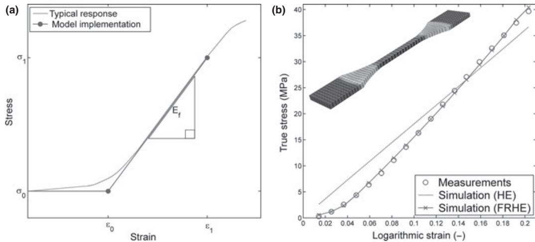
Fig. 4. (a) Typical mechanical response of collagenous skin in tension (red curve) with the implemented response in the present skin model (blue curve). (b) Geometry for a tension measurement with the experimental response (38) to test the suitability of the hyperelastic (HE) and the fibril-reinforced hyperelastic (FRHE) skin models. The mean absolute error between the experimental measurements and the FRHE model was less than 0.3%.
